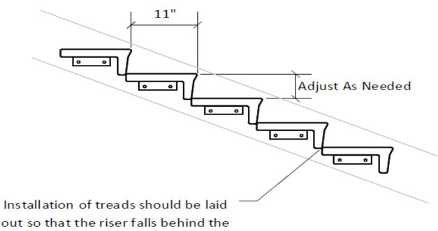
tread below to allow for height adjustment as needed.
