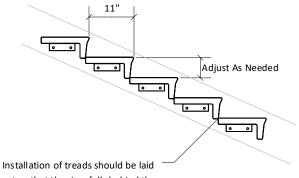
Installation of treads should be laid out so that the riser falls behind the tread below to allow for height adjustment as needed.
